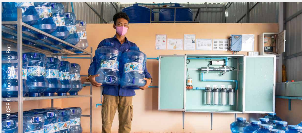
Worker On An stands next to the UV filtration system with freshly filled bottles, ready to be sealed before delivering to customers in Kouk Pou commune, Cambodia.
